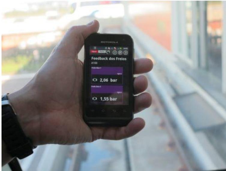
Nunes monitoring pressure on brake's hydraulic system of Aeromovel using his cell phone via Elipse Mobile
